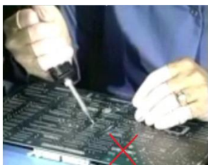
用力将烙铁向下压
